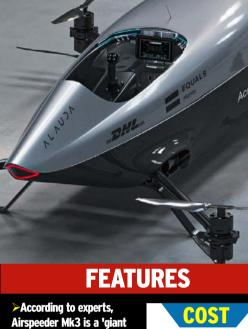
➤ According to experts, Airspeeder Mk3 is a 'giant technical leap forward, as it includes a suite of technologies never seen in an electrical flying vehicle before ▶This includes LiDAR and Radar collision avoidance systems, creating a 'virtual forcefield' around the craft, a carbon fibre frame and fuselage designed for strength, stiffness and lightweight properties Compared to the Mk2,
